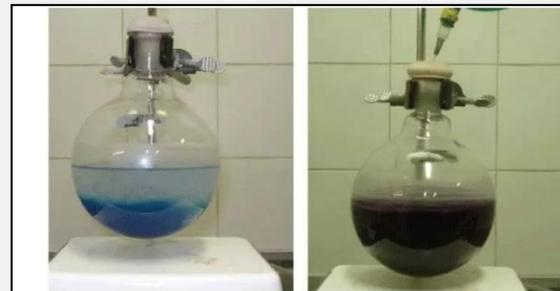
Figure 15. The benzophenone-Ketyl-Ni indicator in action: Color change in THF as soon as stirring begins (on the left) and THF under Ar (on the right).
